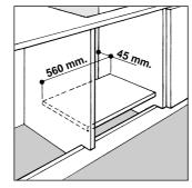
The panels of the adjacent cabinets must be made of heatresistant material. In particular, cabinets with a veneer exterior must be assembled with glues which can withstand temperatures of up to 100 °C.
